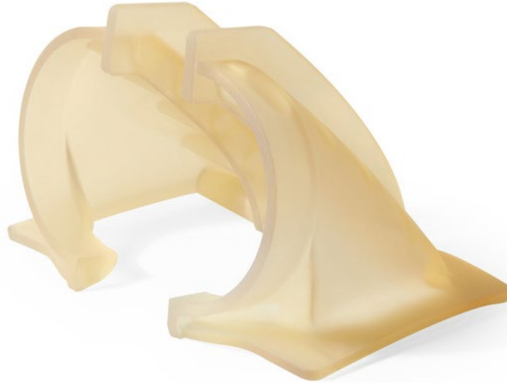
The two-parts mold printed with High Temp Resin.
