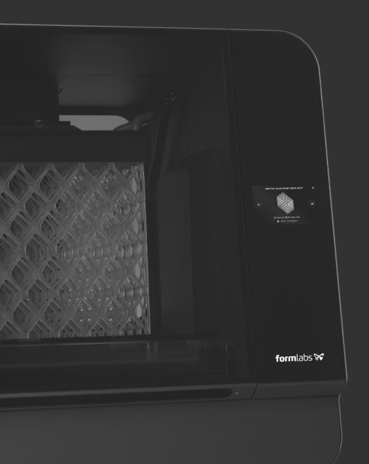
The Form 3 and Form 3L are powered by a new 3D printing process called Low Force Stereolithography (LFS). LFS 3D printing uses a flexible tank and linear illumination to turn liquid resin into flawless parts. Inside the Form 3 and Form 3L is a completely redesigned optics engine, the Light Processing Unit (LPU), which contains a system of lenses and mirrors to deliver accurate, repeatable prints.
