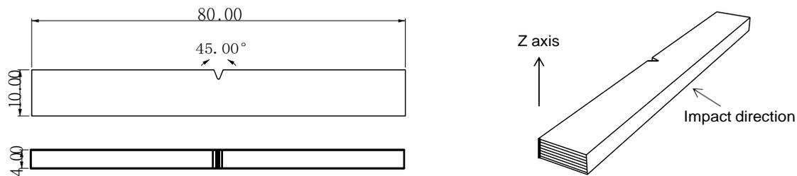
Fig 3. Impact testing specimen
